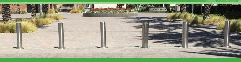
Calpipe Security, located in California, is proud to offer an industrial line of surface mounted base plate bollards manufactured from the highest quality ASTM A53 carbon steel or 300 series stainless steel. Base plate bollards come in a variety of diameters and offer a quick and easy bolt-down installation providing an affixed physical barrier as well as a vehicle deterrence.
