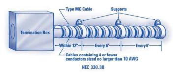
As noted, AC and MC cable support requirements are waived when the cable is fished. This is a major advantage of AC and MC cable in remodeling work over other wiring products that cannot be fished.
