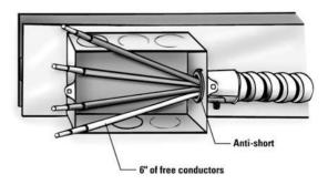
MC cable installed in a box with 6 inches of free conductors left for connections or splices.
