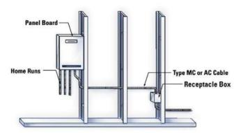
AC & MC cable is available on reels and in coils. If using a reel, simply draw the cable from the end of the reel. If using a coil, draw the cable from the center of the coil to prevent kinking.
