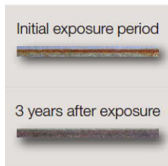
Appearances of cut edges after salt spray test (Thickness: 3.2 mm, coating weight: 120/120 g/m 2 , untreated)
