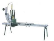
For sizes 2-1/2" to 4" hydraulic benders are available from Calbond. Greenlee 881CT is recommended with shoes designed specifically for PVC coated conduit.
