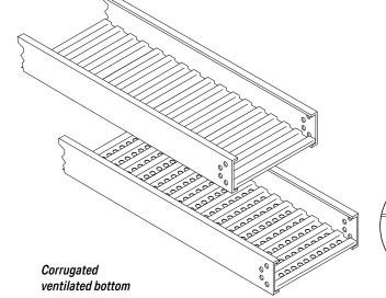
Corrugated bottoms have 1" wide ribs on 2" centers. Optional ventilation holes in the valleys of the corrugations are 11/16" diameter on 1" centers. Free passage of air through the openings results in a 68% open area.
