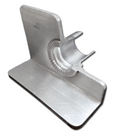
Cold swaged connections create one of the most rigid tray systems in the industry. The swaging process does not affect the temper and strength of surrounding metal the way that traditional welds do.
